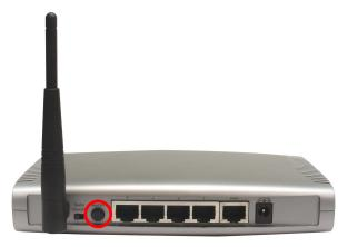
Note: Depending on different type of routers, you may have to push the WPS button on the router first, then push the WPS button on the adapter. Please refer to the router's manual and make sure the WPS session is activated. C) The router will now start to synchronize the encryption settings with the wireless adapter. The connection will be established in few seconds. Continue to Step 3.5.
